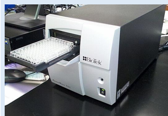
Fig 8A: Typical microplate reader used in research labs. It has the footprint of an office laser printer. Using 96-well microplates tailored for different types of assays, one can determine the levels of biologicals such as insulin, cholesterol etc., in a few microliters of samples accurately within minutes. Image: Licensed under the Creative Commons Attribution-Share Alike 3.0 Unported.
